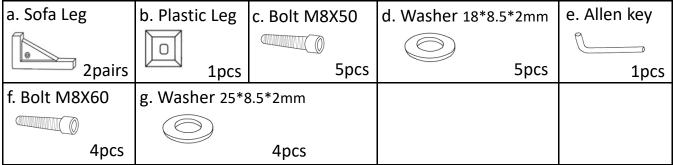
Step2: Tighten the pairs of sofa legs (a) to the bottom of 2-Seater with bolts (c) and washers (d) by Allen key (e).
