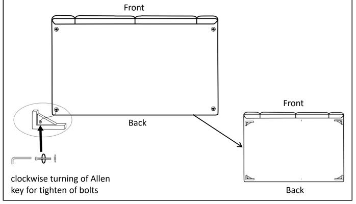
Step3: Tighten the plastic leg (b) to the bottom of 2-Seater with bolts (c) and washers (d) by Allen key (e).
