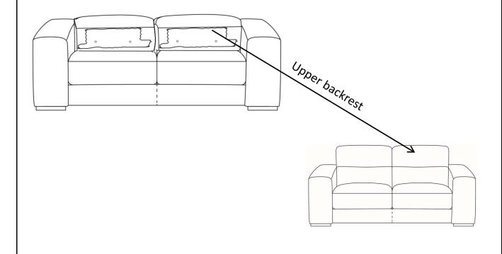
Step5: Tighten the upper backrests to the lower back of 2-Seater with bolts (f) and washers (g) by Allen key (e).
